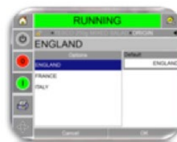
Selection Lists When variable data has to be entered, selection lists remove need for keying
