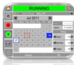
Date Logic Inbuilt control of dates and date offsets reduces risks of date entry errors
